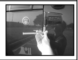
4. To install Tube Doors, lightly lubricate the tube door hinge pins. Position the hinge pins directly above the hinges. Slowly lower the hinge pins into the door hinges. If the hinge pins do not fully seat, slowly rotate the door back and forth until hinge pins fully engage. Install torx nuts removed in the previous step.
