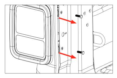
2. Carefully pull the tail light away from the vehicle. Unplug the tail light by sliding red tab first. Then press down on gray tab and gently pull plug from the tail light.
