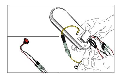
6. Connect wire harness to the factory wire harness. Align the pins on the tail light mount to the rubber grommets on the vehicle. Gently press tail light mount until you feel it click into place.
