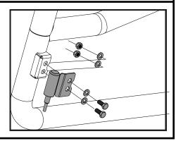
4. To install Tube Doors, lightly lubricate the tube door hinge pins. Position the hinge pins directly above the hinges. Slowly lower the hinge pins into the door hinges. If the hinge pins do not fully seat, slowly rotate the door back and forth until hinge pins fully engage. Install torx nuts removed in the previous step.
