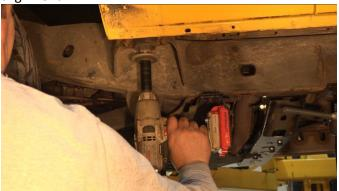
Begin cutting the bracket off, while taking note of its original location, and avoiding damage to the bushing.
