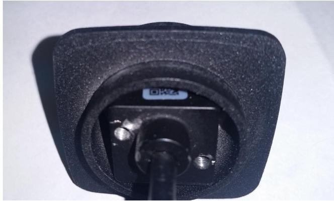
4. Tighten the (2) Allen screws back tight. Apply Z-tech to the back of the camera where the Allen screws are and on the insides on the camera housing.
