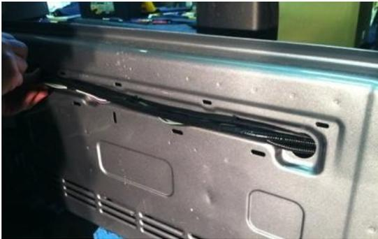
**Step 11:** Use supplied Wire Ties to secure Chassis Harness to fabric factory wire cover. CAUTION: Leave enough slack to allow gate to open fully.
