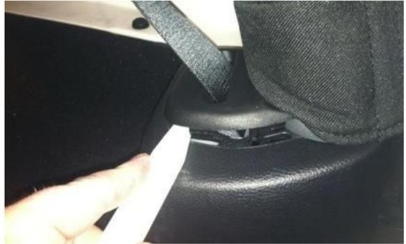
**Step 14:** Using a plastic trim removal tool, remove rear access panel to expose 10mm bolt, and remove bolt.
