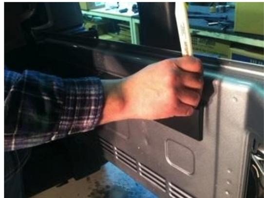
**Step 8:** Pull harness through the rear gate openings.
