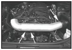
Step 23 Install the intake tube into the flex coupler first then align the mounting bosses. Once in the desired location fasten it securely in place at the flex coupler and the two mounting bosses with the supplied hardware.
