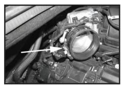
Step 22 Install the coupler on the throttle body and secure the boot in place. Install a second clamp but do not tighten at this time.
