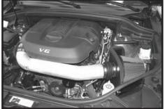
Reinstall the engine cover. Make sure that all clamps and hardware are fully tightened. Reconnect the battery cable, start the vehicle and let it warm up. Shut off and inspect the installation once more for any loose clamps, wires, or hardware. Test
