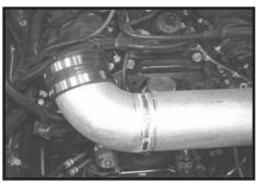
Step 24 Install the coupler on the end of the tube until the tube is flush with the coupler. Do not fasten the clamps at this point; this will be done in the next step.
