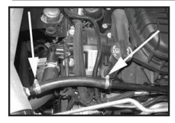
Step 28 Reconnect the factory breather line to intake tube with the provided hose. Fasten it securely in place with the supplied clamps.
