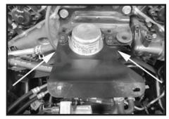
Step 10 Install the provided intake tube bracket onto the air injection pump mounting studs, reinstall the air injection pump and secure it with the nuts removed in Step 9.
