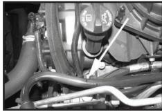
Step 27 Measure the crank case vent tube 5" from the end and then cut off the end.
