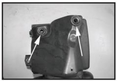
Step 13 Remove the factory grommet from the air box. This will be reused on the next step.
