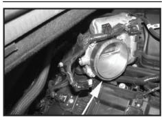
Step 21 Install the throttle body adapter ring onto the throttle body.
