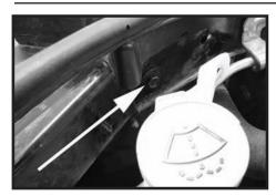
Step 17 Remove the bolt on the core support. This will be reused in the next step.
