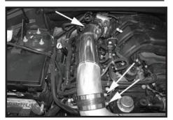
Step 25 Install the small intake tube with the IAT sensor towards the back on the vehicle. Slide the coupler up onto the intake tube that was installed on the previous step. Once in the desired location fasten it securely in place.
