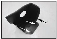
Step 14 Install the rubber bulb seal, this may require trimming to the correct length. Install the grommet removed from Step 8.
