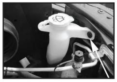
Step 20 Reinstall the panel clip and center pin that was removed in Step 13.
