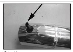
Step 12 Install the supplied grommet into the intake tube then install IAT sensor into the grommet.
