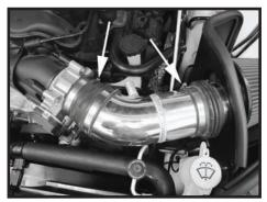
Step 16 Install the intake tube into the flex coupler on the heat shield, and then install the reducer coupler onto the throttle body. Once the tube is in the desired location, tighten all the clamps. The velocity adapter may be rotated slightly once the filter is installed in the vehicle.
