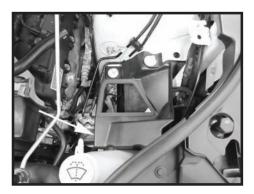
Step 5 Remove the lower air box tray out of the vehicle.
