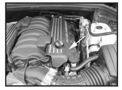
Step 2 Remove the engine cover.
