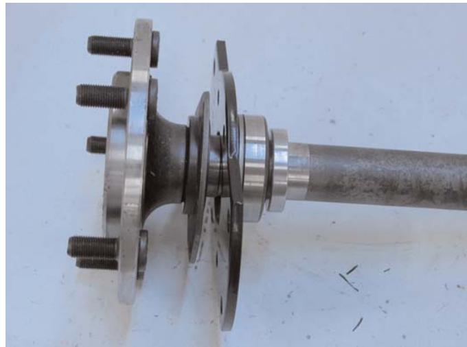
The base caliper mounting bracket must be installed between the retainer plate and the bearing. Those parts are supplied with your new axles not the brake kit. Be sure to check the bracket orientation before pressing the bearing on. The brackets should be clocked slightly towards the front of the Jeep when installed on the housing. Refer to the instructions supplied with your axles for further details and proper procedure for pressing the bearing.
