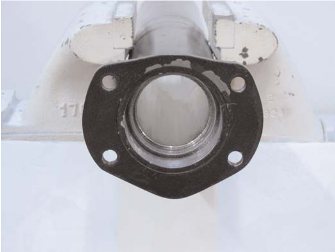
View of axle housing with the axle and brakes removed.
