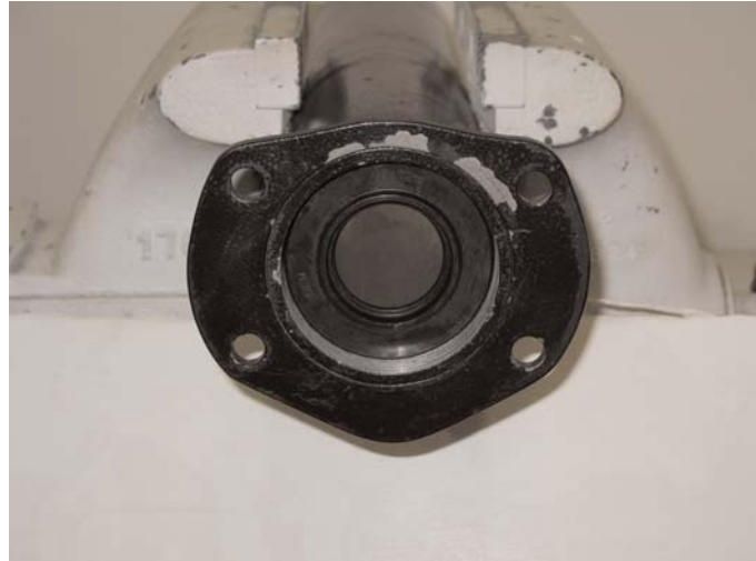
Install the bearing seal supplied with your new axles in the axle housing.
