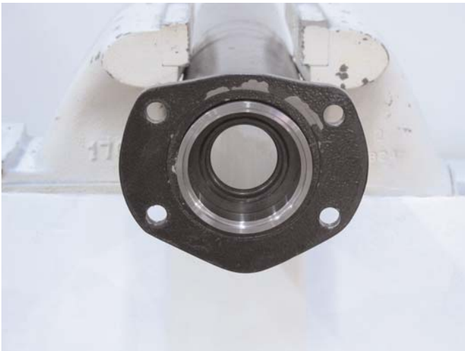
Install the spacer ring supplied with your new axles into the axle housing.
