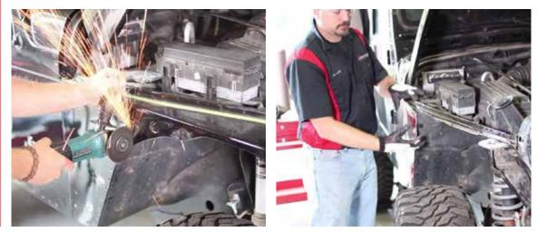
7 Cut front of the fneder right before it meets up with the grill and remove support bracket here.
