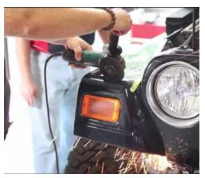
**6** Cut at the just before the inner fender meets the outside of the fender. The second photo is how it should look when you are done cutting.
