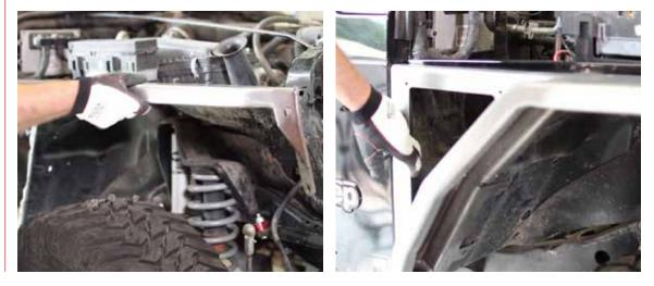
17 Starting with the rear, install the rest of the bolts loosely. This will be 4 13 mm bolts in the rear,
