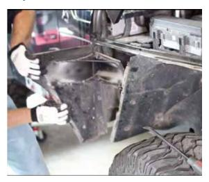
${\bf 9}$  13mm wrench to remove the 4 rear bolts at the body and remove the 4 bolts in the inner fender.
