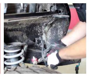
**14** Install new battery bracket using stock fasteners and reuse your old battery tray 5/16 bolts and flange nuts.
