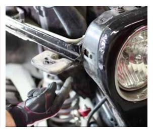
8 Pry back the rear panel like this, so you can get access to the bolts mounting the fender to the body.
