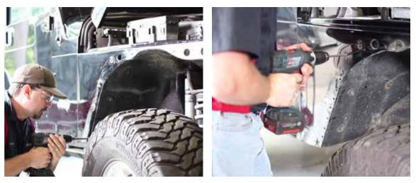
4 Using tape or a marker, mark off an inch out from hood fold on the top of the fender. Now cut along this line using your cutting tool like a cut off wheel on a angle grinder or sawsall.
