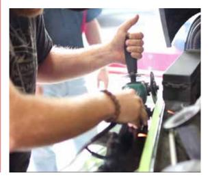
**5** Cut along the front right above the bend. This is just so you can get that front portion out of the way.
