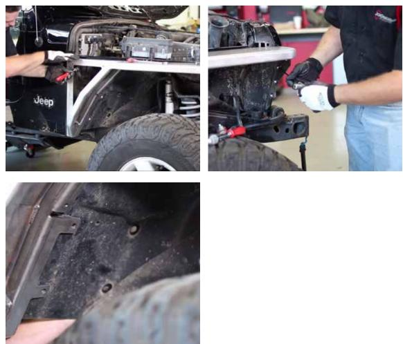
**18** Line up your fenders with your rear body lines and then tighten down one of the rear bolts. For the front you will make sure that you line up with the bottom of the square hole in the grill.
