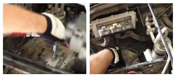
11 Still using the 13mm socket, remove the 6 fasteners holding the battery tray to the bulkhead and then remove the battery tray.
