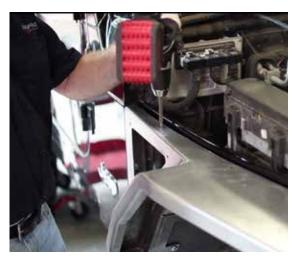
20 Use the 1/4 inch button heads and flange nuts through the new holes that you just drilled. I recommend some RTV if this is your final install or once the new fender is off paint the holes.
