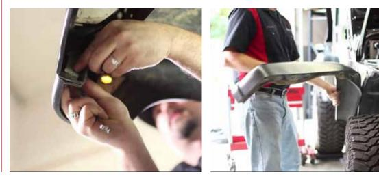
**3** A few inches past the wheel well you will see 10 spot weld dimples going up the outside of the fender. Drill these out with a 5/16th drill bit.
