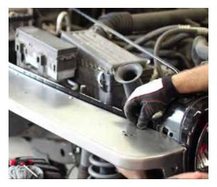
Reinstall the factory latch using the 13mm socket.
