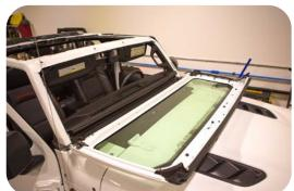
Attach the (4) header clips to the header rail and then reconnect your windshield and wipers.
