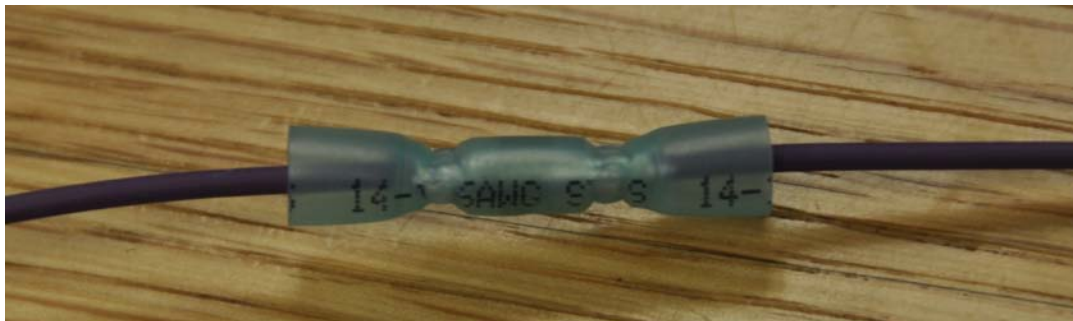
Figure 1. Slide on heat shrink tube before you twist and crimp the wires.
