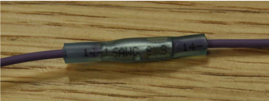
Figure 3: Complete heat shrink splice
