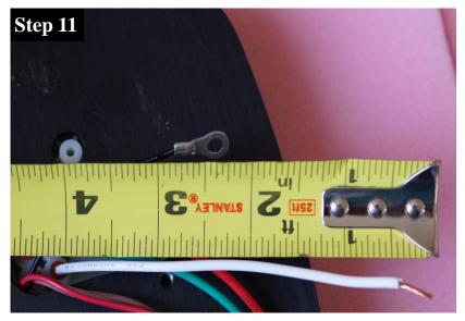
The white wire on the tail light lens must be grounded to the tail light housing. Measure and cut the white wire to 4 inches.
