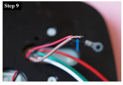
Strip about 5/16" off the insulation for both brown and red wires and twist together as shown in blue arrow.
