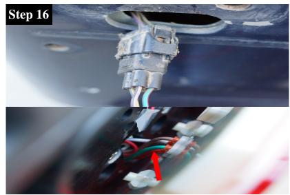
Continue your installation on the driver side of the vehicle. Plug the tail light in and push the wiring back into the Jeep tub.
