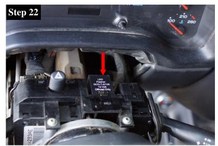
Install the LED Flasher Relay as shown by the (red arrow).
