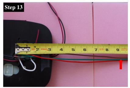
Measure and cut the tail light lens red, brown and green wires to nine inches at the location shown by the red arrow.
