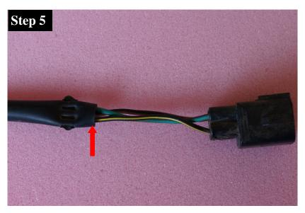
Take the driver side (left) OEM tail light housing and cut the harness plug at the heat shrink crimp area (red arrow).
