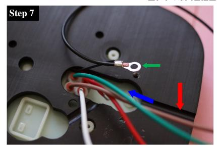
Note: When the lens is installed in the housing the area shown by the blue arrow must be kept clear as the wiring must bend and clear the Jeep tub.
