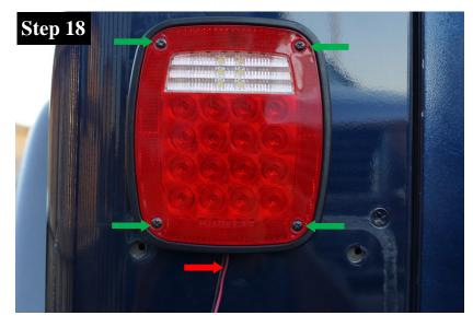
Install (4) #6 - 32 x 5/8" Pan Head Machine Screws (E) as shown in the green arrows. Start all 4 screws before tightening to snug. **Do not overtighten to avoid cracking the tail light lens.**
