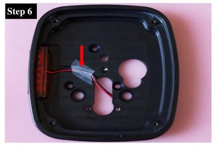
The Tail Light Housing includes a LED side marker light that must be tied into the housing ground plane and the running light power signal. These steps will be performed later on.
