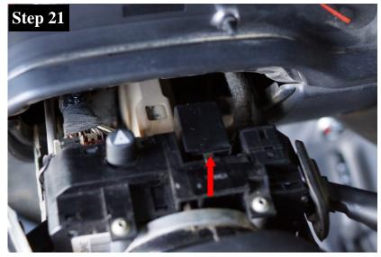
Grab the OEM flasher relay and pull in the direction as shown by the red arrow.
