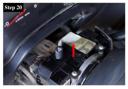
Under the tape is the OEM flasher relay that will be replaced (red arrow).
