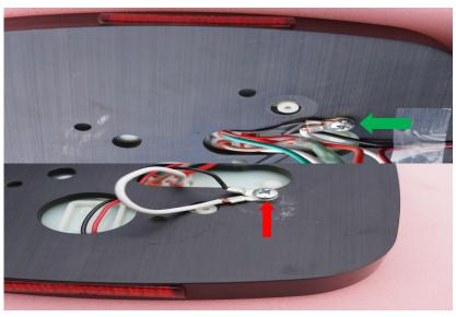
Crimp a #6 Ring Terminal to the white wire and install both the side marker, license plate lighting and tail light lens grounds to the housing using (1)  $6 - 32 \times 1/4$ " Pan Head Machine Screw (F) on the threaded hole closest to the side marker lens.
