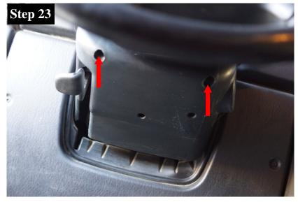
Reinstall the steering column cover and two screws previously removed.
