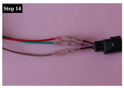
Strip 5/16" off the insulation of the tail light lens wires and OEM plug wires.
