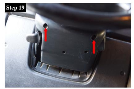
To install the LED Flasher Relay remove the two screws as shown by the red arrows.
