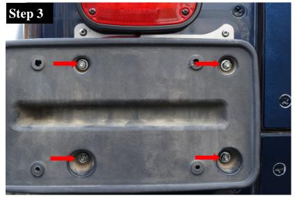
Reinstall the OEM Stock License Plate Holder using (4) #10 Stainless Steel Washers (D) and (4) 10-32 Nylon-Insert Hex Locknuts (B) (red arrows). Snug only to prevent the studs from spinning.
