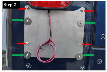
Install the License Plate Relocator (A) as shown with studs facing outwards.
