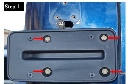
Remove the four screws that hold the license plate mount (red arrows).
