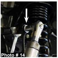
28. Connect the OEM front track bar to the frame using the OEM hardware & a 21mm socket / wrench. (See Photo # 4) **Note:** Slightly turning the steering wheel will help align the OEM front track bar with the frame mount.
