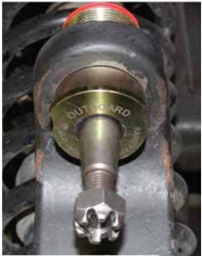
Ensure outer lip is facing outboard.
