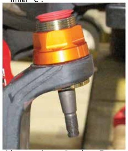
Press upper ball joint into place using HD ball joint tool. Ensure bottom face sits flush against inner "C".
