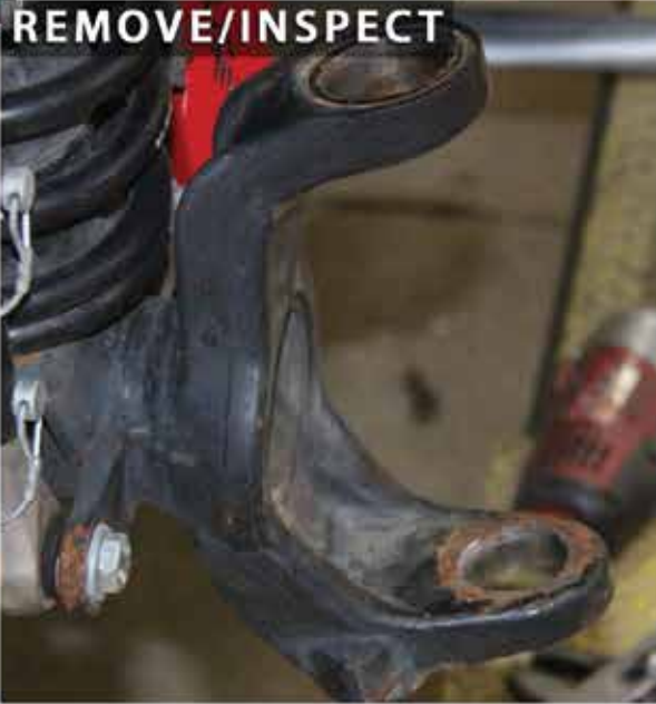
Remove old ball joints. Clean and inspect upper and lower ball joint holes in inner "C".
