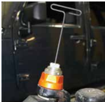
Tighten using the supplied T-handle wrench until cap stops turning and wrench flexes (approx 50 INCH/lbs). DO NOT exceed 55 INCH/lbs. Do not use ft/lb wrench.
