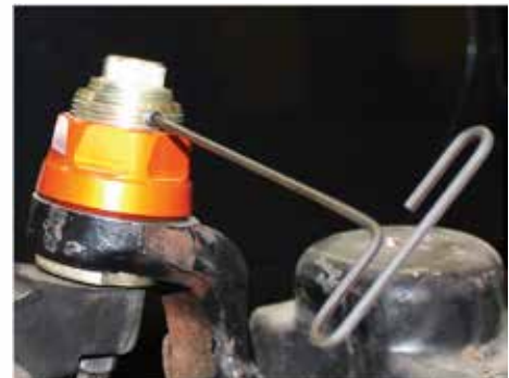
Install 1/4-28 set screw to lock the cap in place, and tighten with supplied 1/8" T-handle wrench. Install upper grease fittings.
