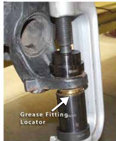
Using the HD ball joint press tool, press lower ball joint up into place.
