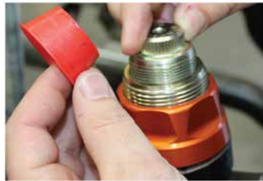
Remove the red caps, and install the load carrying cap by hand.
