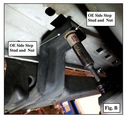
**<u>Step 4</u>**: Carefully remove the **OE** side step from the vehicle. By pulling outward to clear the studs and then down to clear the mounts. (Fig. C)
