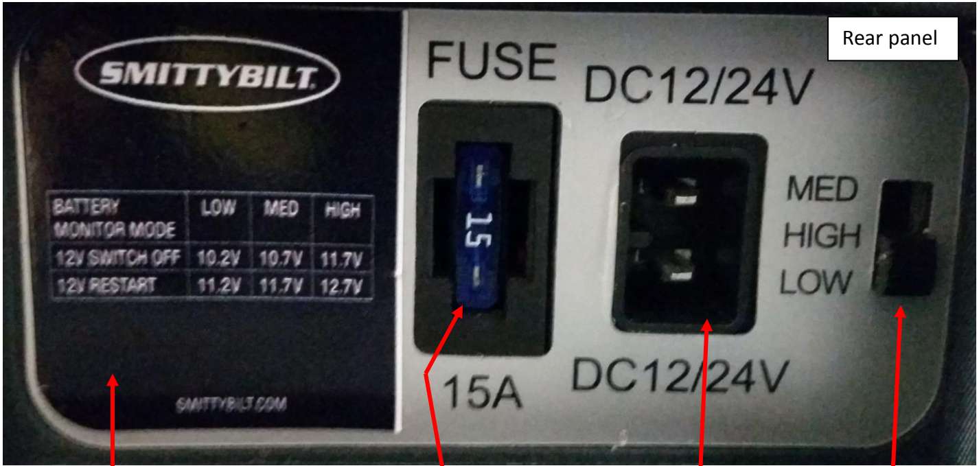
Battery monitor voltage table.
