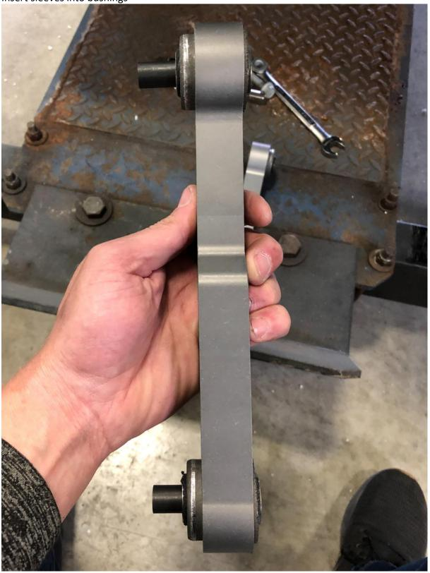
4. Slide fastener through top hole, place spacer between end link bushing and sway bar SPACER FASTENER
