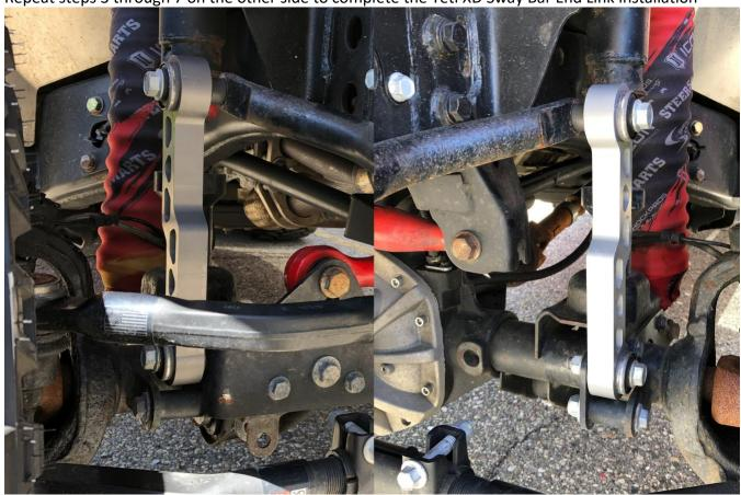
a. Note that this Jeep is equipped with a Top Mount draglink and our trackbar relocation bracket. If you are running a JK/JL w/o a trackbar relocation bracket, mounting location is shown below:
