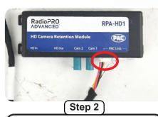
Connect one end of the 18" harness (10P-2-10P-18) into either of the two 10-pin PAC Link ports on the RPA-HD1 interface module. The other end will be connected to the open 10-pin port on the PL1 interface module after mounting the radio unit into the vehicle.
