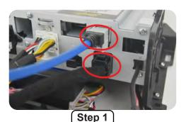
Connect one end of the 8-pin display power harness into the 8-pin port on the Stinger radio module, then connect the LVDS display video cable into the LVDS display port on the Stinger radio module. (Both of these cables are provided in the Stinger radio box.)
