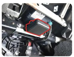
Note: Installation of the chime speaker is only required in vehicles with safety group features.
