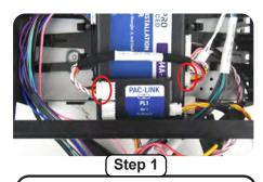
Connect one end of the 6" harness (10P-2-10P-6) into the 10-pin expansion port on the CH4A-JW18 interface module. then connect the other end into either of the two 10-pin ports on the PL1 interface module.
