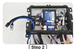
Route the display harness and cable through the front opening of the main radio module mounting bracket.
