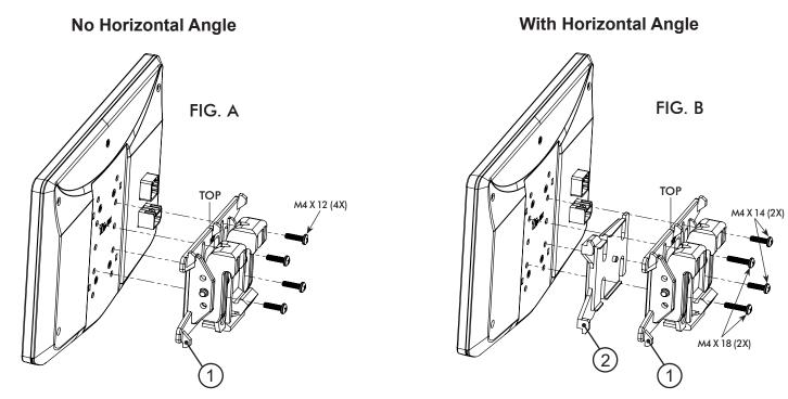
Always ensure TOP indicator on the Clamp Assembly is facing UP.
