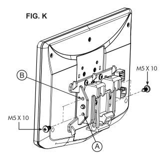
**VERTICAL TILT**: Use **Hole A** for no vertical tilt or **Hole B** for 8 degrees of vertical tilt. Insert a M5 X 10 on each side of the clamp assembly at desired tilt.
