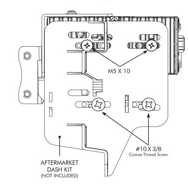
Note: If there is a depth issue with the radio module in the top position, move it to the bottom location by inverting the mounting bracket assembly. (FIG. I)
