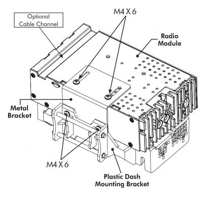
Single DIN Applications: For Single DIN installations, the *Plastic Dash Mounting Bracket* will be mounted in the dash kit the dash kit and the *Radio Module* will be mounted remotely. Before beginning the installation, determine where the *Radio Module* will be installed and make sure the Display Cables are long enough. Longer, 5 foot cables are available (SE-1501 & SE-1502).
