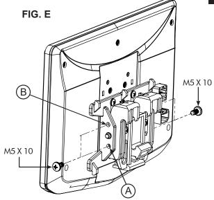
**VERTICAL TILT**: Use **Hole A** for no vertical tilt or **Hole B** for 8 degrees of vertical tilt. Insert a M5 X 10 on each side of the clamp assembly at desired tilt.
