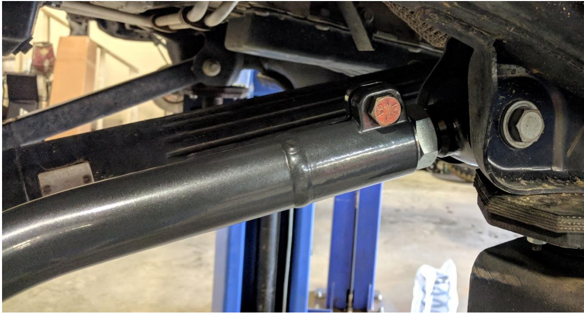
Figure 4. Control Arm Correctly Installed (Frame Side Shown)
