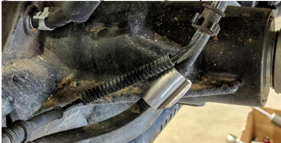
Figure 3. Brake Line Trimmed
