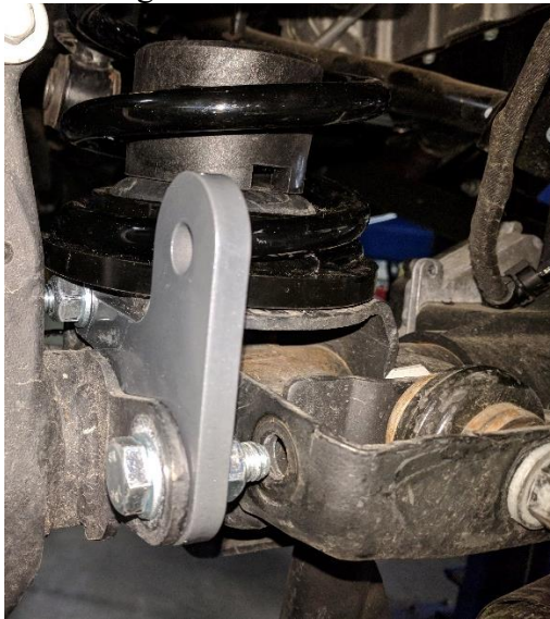
Figures 4 and 5. Correctly Installed Brackets (Passenger side on Left, Driver on Right)
