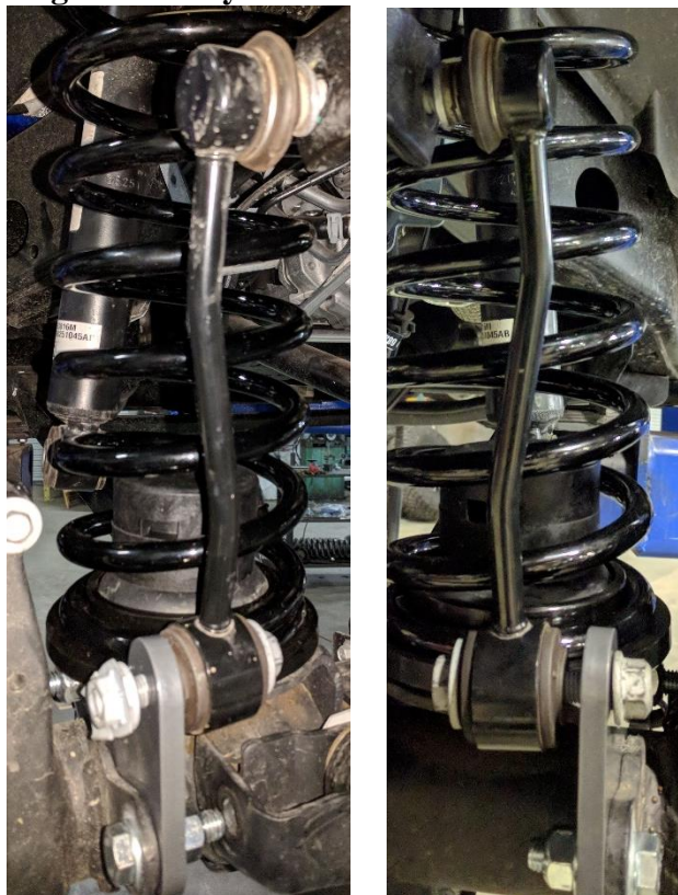
Figures 7 and 8. Correctly Installed Sway Bar Links (Passenger side on Left, Driver on Right)
