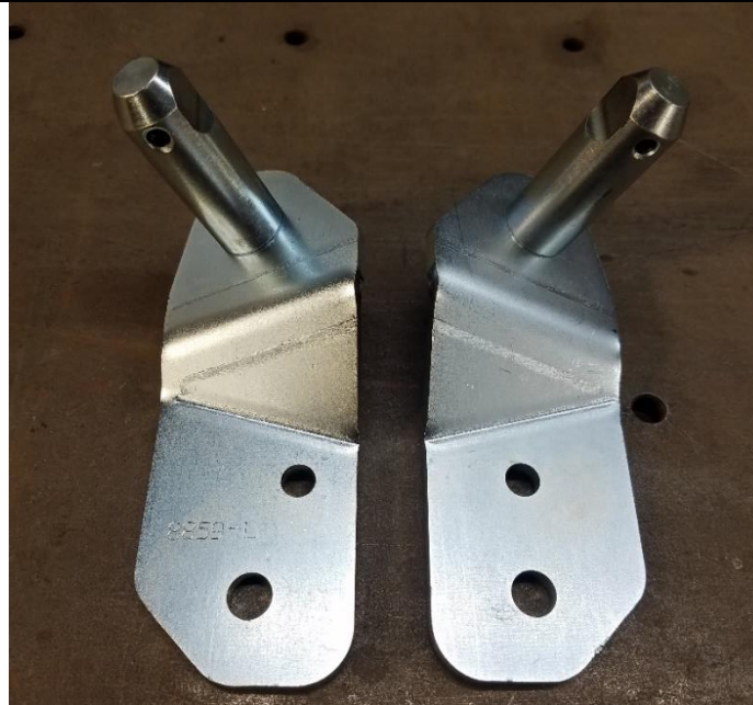
Figure 8. Disconnect Pins Installed into the Brackets.
