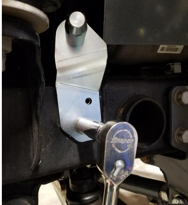
Figure 10. Installing the Lower 3/8" Bolt Through the Frame (Driver's Side)
