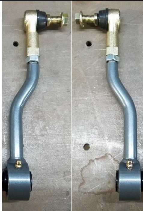
Figure 2. Setting the End Links to the Same Length
