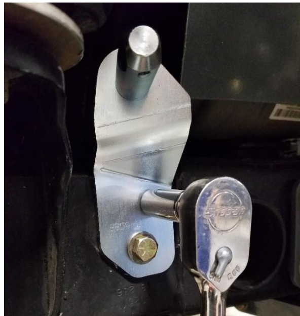
Figure 11. Installing the 5/16" Self-Tapping Bolt in the Upper Hole (Driver's Side)
