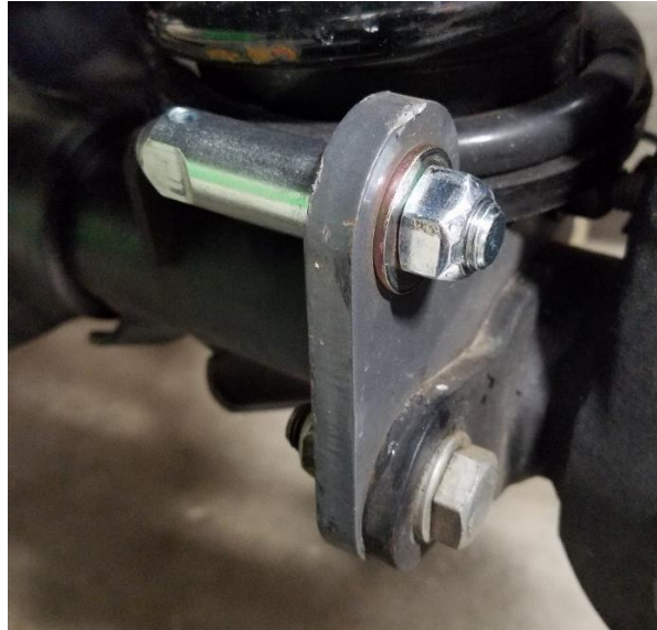
Figure 5. Disconnect Stud Installed in Relocation Bracket
