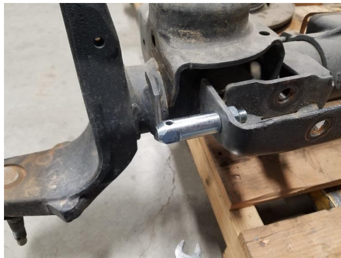
Figure 5. Disconnect Stud Installed on Factory Track Bar Mount
