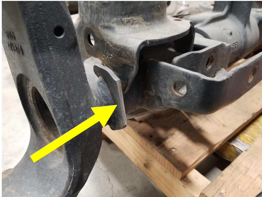
Figure 1. Removing Outer Passenger Side Sway Bar Tab
