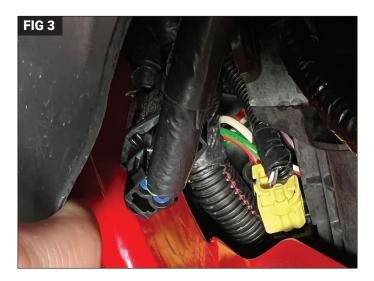
Locate the wiring harness for the running lights and side markers. Release the clip and pull apart. (Fig 3)
