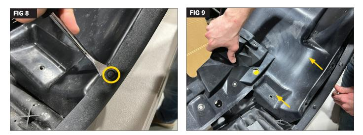
Disconnect the inner fender liner from the fender flare by using a pry tool between each piece at the plastic retaining rivets and pry out. (Fig 8) Once each rivet has been released, slide the inner fender liner away from the flare. (Fig 9)
