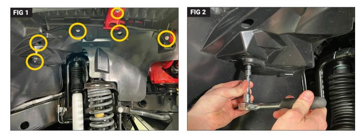
Remove the 6 bolts (circled) holding the fender flares and liners (Fig 1) using a 10mm socket and ratchet. (Fig 2) Retain for reassembly.
