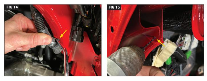
Remove the wiring group from the sheet metal by releasing the retaining clip. This will allow the wiring to move freely and be a little longer to reach the wiring harness a little later. (Fig 14) Using a 7/64" drill bit, drill a pilot hole to be used with a self-tapping screw in Step 8. (Fig 15)
