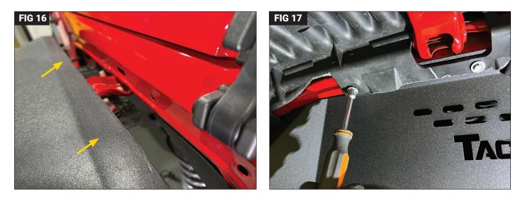
Holding the inner liner and fender flare together, slide the assembly back onto the quarter panel allowing the clips to engage and hold the flare in place. Start with the bolt toward the center. (Fig 16) From underneath begin to replace the factory 10mm bolts to hold in place. (Fig 17)
