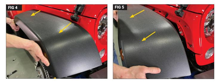
Using even force and hands grasping the edge of the fender flares, pull directly away from the quarter panel. (Fig 4) There will be tension on from the clips and you will find resistance until they release. Some clips my stay attached to the quarter panel. (Fig 5) Remove with a pry tool and reattach to the fender flare.
