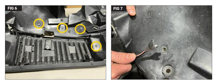
Locate the four retainer clips shown with circles. (Fig 6) Using a pry tool, remove each one. (Fig 7)
