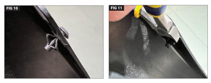
Note that the retaining rivets from the previous step remain. (Fig 10) These can be cut away as they will not be reused. (Fig 11)
