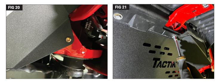
Using the 7/64" drill bit and using the liner as a guide, drill a pilot hole for the remaining self-tapping screw. Insert and tighten the self-tapping screw. (Fig 20) Tighten remaining 10mm bolts to secure the fender liner and flare. (Fig 21)
