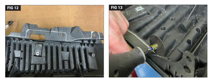
In order to perform Step 7, you will need to draw a line on the inside of the fender, and then cut along the line you drew. IT'S VERY IMPORTANT TO DRAW THE LINE BEFORE YOU BEGIN TO CUT! Using a marker or a paint pen, draw the line as shown in FIG 12. Next, using a cutting tool, carefully cut along the line that you drew. This line may need to be adjusted slightly after cutting. (Fig 13). **Remember:** You can always remove more material, but you can't add it back on.
