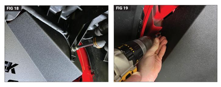
Insert and tighten the bolt on the structural brace to secure the fender and liner to the vehicle. (Fig 18) Insert and tighten the self-taping screw into the pilot hole drilled previously. (Fig 19)
