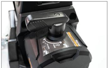
There are two positions of the clutch handle. The Clutch is either "engaged" or "free spooling". The clutch allows the operator to manually engage or disengage the spooling drum from the gearset using the clutch lever.
