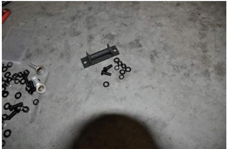
9. Install bracket on to the tire carrier. This bracket will line up with the “U” shaped spot on the tailgate plate. To line up, loosely bolt up the bracket and close tailgate. Tighten the bracket once you aligned it with the “U” shaped area of the tailgate. Hand tighten only.
