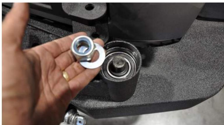
7. Bolt in the composite "U" shaped piece on to the tailgate plate using supplied nuts, bolts, washers and split-washers. Firmly hand-tighten.
