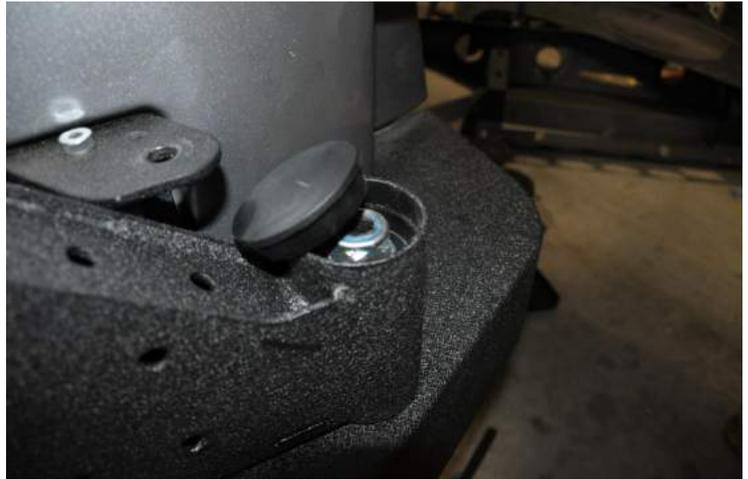
13. Locate the spare tire inner mounting bracket and nuts and bolts for it. See picture.
