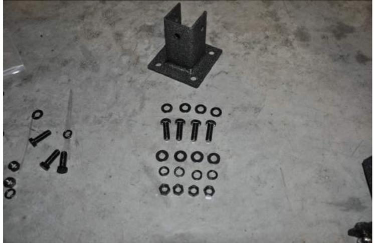
14. Bolt to the outside of the tire carrier. In order to make sure your tire will clear the bumper use a helper to lift spare tire up to see how far up to mount the bracket. Torque the bolts to 25lbs. Note: To minimize shaking you want the spare to be at the lowest level necessary to clear the bumper.
