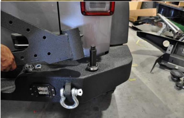
6. Drop the new washer on top of the second bearing and spin on the large nylock nut. In order to tighten the carrier you will be tightening both the top and bottom of the axle shaft at the same time. You can use a socket for the top but will need a wrench for the bottom nut. Note: Hand tighten only!
