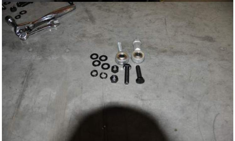
11. Screw the heims together and bolt the female end to the carrier. To set the other end length, close the tailgate and tire carrier. Rotate the male end of the heim to lengthen or shorten to line up with the bracket on the tailgate plate like shown in picture. Open tailgate and rotate the male end of hiem 1/2 turn tighter and bolt up to tail gate bracket. Torque bolts for heims to 20lbs.
