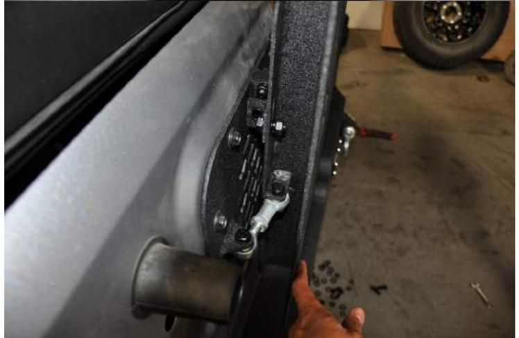
12. Install the new rubber cap over the axle bolt bearing area on tire carrier. This piece will help keep the bearing clean and smooth.
