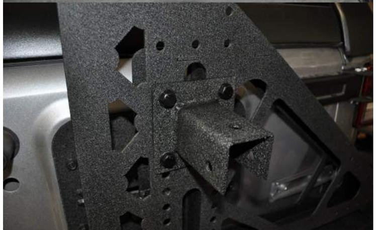
15. Bolt the outer portion of the spare bracket to the inner part. Keep the bolts a little loose. With the outer all the way extended, place the spare on it and push tire till tire touches the carrier. Remove tire. Slide outer part of bracket in extra 1/4 inch and torque bolts to 40lbs. Re-install tire using the lug nuts supplied with our kit. Torque to 50lbs.
