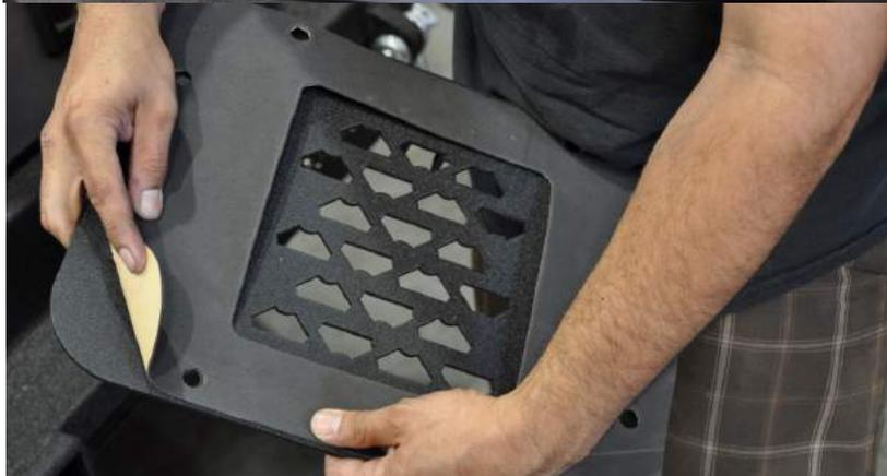
4. Attach the new tailgate plate using the factory hardware. Torque the bolts to 15lbs. Make sure the plate orientation is the same as pictured.
