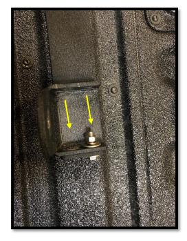
4. Move the lower bottom bracket in place. In the side of the JT, you have two holes, a threaded and non-threaded. Using the supplied hardware, loosely thread lower bottom bracket into side of bed.
