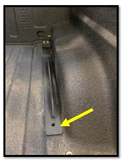
9. To mount tire, insert threaded post into carrier from the exterior facing to the interior. Place tire onto post and place cone facing wheel followed by round plate and T-handle. As you are tightening the T-handle, place your foot on the wheel and press tire into bed as you tighten the carrier.
