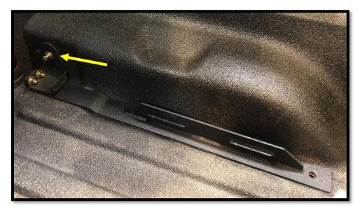
5. Next, install the two slide brackets into the rail. You will need to use the large access hole in the front to fit the mounts into the rail. Ensure you use supplied hardware as shown in the image. These will be tightened later to keep slide mounts into place.
