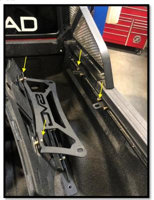
8. Maneuver carrier into desired position and tighten all hardware. Ensure to tighten slide bracket bolts to lock position. After ALL hardware it secure, mark hole at end of lower bottom bracket. Drill ½" hole and secure with bolt and nut. (Drilled stability hole recommended for 35" or larger tires)
