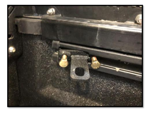
6. Using the provided hardware, mount the main carrier to the lower bottom bracket. Keep carrier loose at this point.
