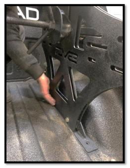
7. Once carrier is loosely attached to the lower bottom bracket, attached the rail bracket to the carrier and the two slide brackets.
