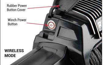
**NOTE:** The wireless remote is designed to work within a range of 10' from the winch but may work at farther distances depending on physical obstructions and other conditions. It is not recommended to use the wireless feature from the cab of your vehicle. If you choose to winch from the cab, use the wired option for safety.
