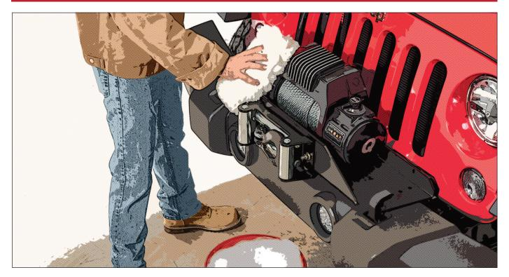
Do not direct very high-pressure water at your winch. Use low-pressure (normal) car wash soap and water to clean your winch. With the remote control disconnected and the protective boots covering the remote control socket and Power Button sockets, wash normally with your vehicle. During winter exposure to road salt, wash the winch as soon as possible to avoid corrosion. Always wash per the recommendations above.
