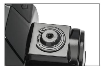
Rotate Clutch Handle to the "FREE SPOOL" position to reveal the set screw that holds the handle in place. Using a 2.5 MM Allen wrench, back out the set screw until the Clutch Handle lifts off but do not remove the handle at this time. Rotate the clutch selector to the "ENGAGED" position. You may remove the Clutch Handle now and keep it in a safe place. We suggest keeping the Clutch Handle somewhere in the vehicle.
