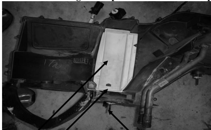
Drain reservoir Hole for drain Drain
