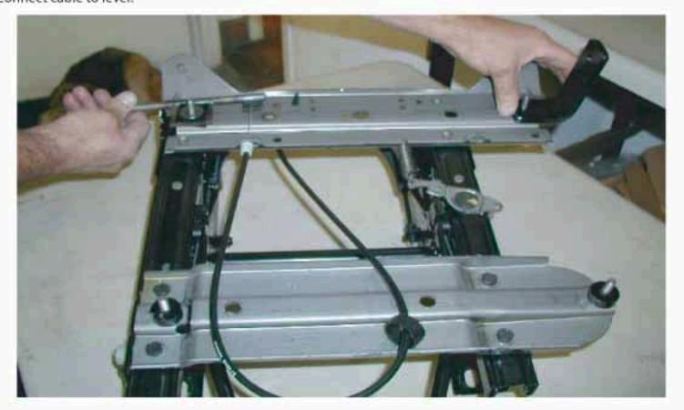
Step #9 Then mount seat over top of studs using the provided nyloc nuts and washers.
