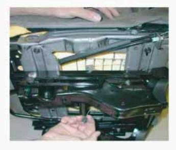
Step # 3 - Remove the cables from the cable bracketpassenger seat, inside rear.
