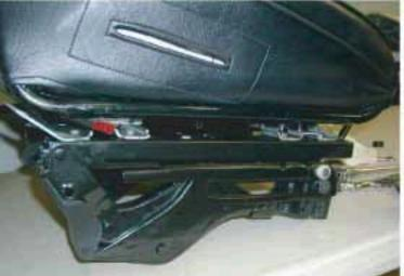
Step # 10 Install seat belt reciever/bracket using the factory bolts. Install assembled seats and risers back into vehicle.
