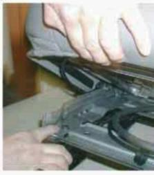
Step # 6 - Remove the top cable with the black end completely from the riser and discard.
