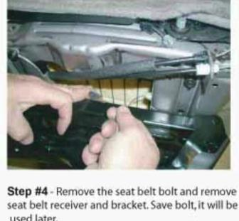
seat belt receiver and bracket. Save bolt, it will be used later.
