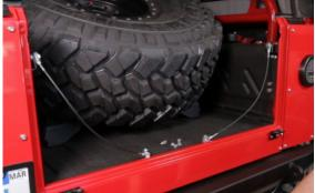
$oldsymbol{8}$  Install the tailgate to the hinges using the 5/16" button head bolts and flange nuts.
