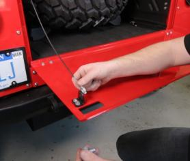
Your latch may come assembled already. Check to see if it is in the following configuration. From bottom to top: locking plate, nut, lock washer, latch pin, lock and a nut on top. If it is not installed, go ahead and assemble in this order. Then bolt the latch in plate using the backing plate, lock washer and bolt.
