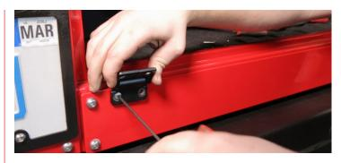
Using a 9/32" drill bit, drill the holes for the upper cable brackets. The positioning of these may depend on your Jeep but the goal is for the cables to be tight when the tailgate is laying perfectly flat. We recommend 10.5" up from the floor, and 1" in from the inner edge of the tub to the rearmost bolt. Go up from beneath the tub or remove the tail lights to gain access to put the flange nuts on. Use the longer 1/4" button head bolt towards the front of the Jeep.
