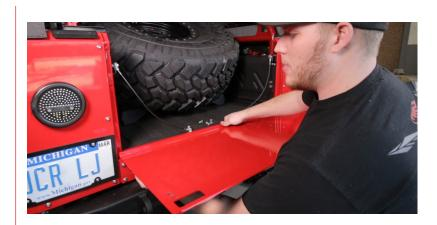
Install the lower cable brackets onto the tailgate using the 1/4" button head bolts. Then bolt the cables to the inside edge of the brackets.
