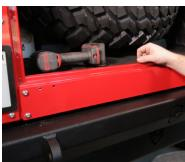
4 Using a 9/32" drill bit, drill through the plate and through the body. You will need to ream the holes out slightly, just large enough so that the smaller nutserts fit snug. Remove the lower plate again. Install the smaller M5 nutserts and reinstall the lower plate.
