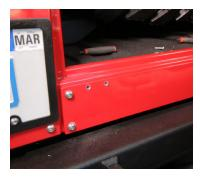
5 Install the hinges using the M5 button head bolts.
