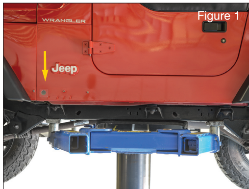
Removal or modification of the fender flair extension may be required when installing the rocker guard(#12004.3202) BUT NOT THE SIDE ARMOR (#12004.3212). (Figure 1)
