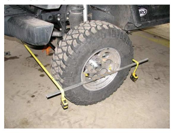
Utilizing a pair of straight edge materials (aluminum C-channel shown, available from most hardware stores) and a pair of bungee cords, attach the straight edges to the wheels as shown. Take care to not bend/deflect the straight edge with the tension of the bungees, but yet you need to have enough tension to keep the straight edges in place.
