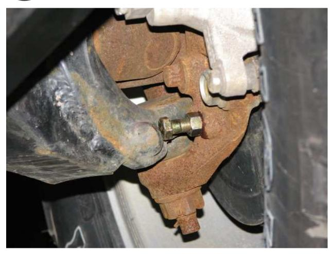
Steering stop adjustment. There are a pair of 3/8" x 1.25" bolts supplied in the kit, with nuts, these are to be used to replace the stock steering stop bolts. Due to the new geometry of the tie rod ends, the outside tire (left tire on a right turn) will turn farther than previous, so we need to adjust the stops to keep the tire from contacting the suspension components.
