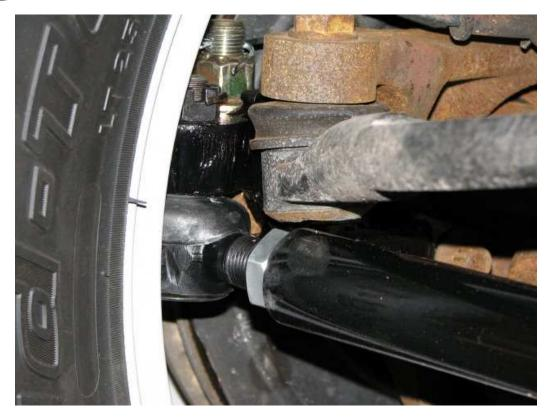
Draglink adjustment. At full turn to the right, the draglink tie rod end, shown in the above picture, may contact the tie rod depending on the rotation of the draglink.
