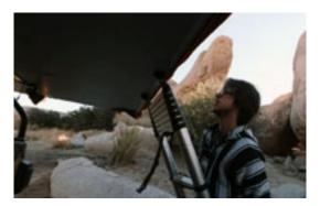
4. Grab the black nylon strap attached to the top of the shell (you may need the help of the rods of the canopy to reach the strap). Pull down on the strap to close the hard shell.
