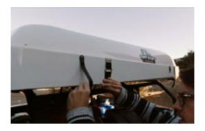
2. With one hand, push up the hard shell handle. The gas struts will open the rest of the tent on its own.
