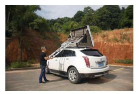
6. After the extension floor has been lowered, secure the ladder by bringing the top rungs up until they are locked into place. \*Do not collapse the bottom rungs\*
