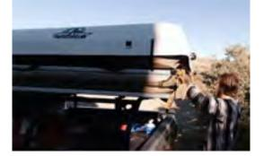
6. Pull down the straps, and securely fasten the fastening and reinforced straps.
