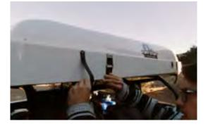
2. With one hand, push up the hard shell handle. The gas struts will open the rest of the tent on its own.
