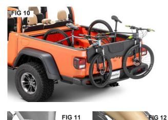
Loading the bikes. Place the bikes on the tailgate, starting from the left side first. Make sure your bike's disc (where applicable)brake is facing out from the pad and the wheel is tilted out where possible. Position the bicycles so the front forks are resting on the bike pad and the back wheels touch the bed of the truck (FIG10). Use great care when placing the bikes inside the rear of your vehicle as not to scratch your truck bed with the pedals.
