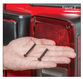
difference when removed. The larger screws (thicker) go on the outside of the Taillight housing where the smaller screws go on the inside (Fig 2). Set aside the original screws, as they will not be used with Euro-Guards.
