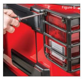
hole of the taillight and repeat the procedure this time using the **smaller** screw and a Lens/Euro-Guard Spacer (Fig 4).
