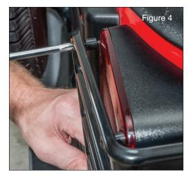
screw on the inside of the Euro-Guard (Fig 3). Install the **larger** screw into the **outer** top screw hole on the light housing itself and tighten only slightly. DO NOT Tighten all the way at this time. Next, move to the upper **inside**
