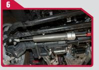
Adjust stabilizer length by turning the wheel until the steering stabilizer eyelet fits into the bracket and aligns with the bracket holes. Using the softest setting to make the adjustment easier
