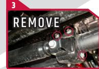
Remove the three factory steering stabilizer bolts on the axle bracket Retain factory hardware
