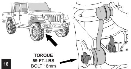
NOTE: DO NOT TIGHTEN THE CONTROL ARM BOLTS UNTIL THE JEEP IS ON THE GROUND
