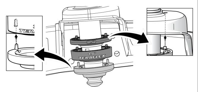
NOTE: IF YOU PLAN ON FREQUENTLY CARRYING HEAVY LOADS WE RECOMMEND ONLY INSTALLING THE 1" SPACER FOR A MORE LEVEL APPEARANCE WHEN LOADED.
