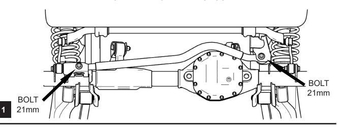
ADJUST THE NEW TRACK BAR TO THE APPROXIMATE LENGTH NEEDED TO CENTER THE AXLE UNDER THE JEEP
