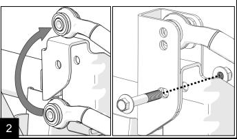
Install track bar bracket with the provided M12 bolt and M12 nut into the holes just drilled.
