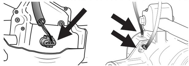
**RECONNECT PLASTIC RETAINERS FROM WIRING OR HOSES AS NEEDED.**
