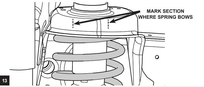
REMOVE THE UPPER SPRING ISOLATOR AND CUT OFF THE TWO ALIGNMENT PINS
