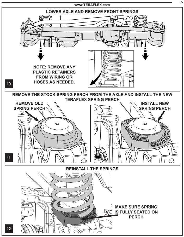
WITH SPRINGS REINSTALLED LOWER THE JEEP TO RIDE HEIGHT. IF THE SPRINGS APPEAR TO BE BOWING OUT YOU MAY NEED TO MODIFY THE UPPER SPRING ISOLATOR AS SHOWN IN STEPS 13-16.
