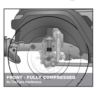
In order to address these fender differences, TeraFlex designed a proprietary modular bump stop system, which can be adapted to fit several different lift height and tire size configurations.
