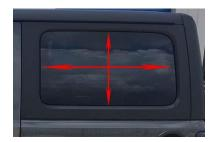
• Locate and mark the center point of the side rear window armor guard. Run a thin tape from top to bottom and from side to side.
