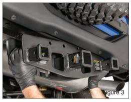
plate (FIG 2) and retaining washers. These are no longer needed. Install the hitch over the rear cross member (FIG 3), then reinstall the 4 factory bolts
