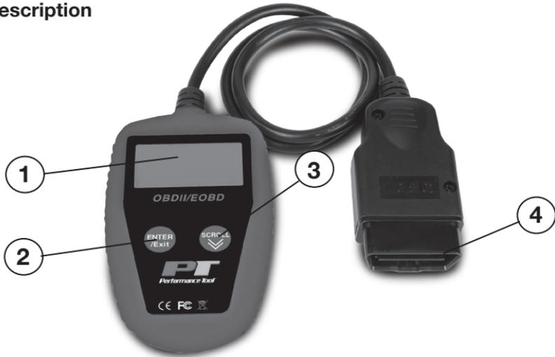
**1. LCD DISPLAY** - Indicates test results. It is a backlit 2-line display with 8 characters on each line.
