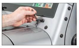
Completely remove both bolts with the supplied T40 Torx Wrench.
