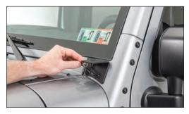
Install the light bracket as shown with the two bolts from the previous step and tighten.
