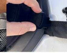
**Connect the 2nd Hook in the Door Limiting Strap Slot**
