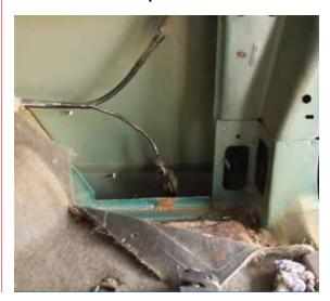
Install the spindle reinforcement brackets by finding the rectangular access hole in the bulkhead located on the passenger side above and to the right of the passenger leaf spring shackle. You will see two holes in the access hole that will need to be enlarged to a 1/2 inch.
