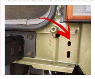
Place the L shaped bracket with the short leg against the two holes that you just enlarged and the long side facing the passenger side. Place the second bracket with the gusset facing the passenger side and the long portion facing up. Insert two 7/16x1 bolts with 3/8 washers through one bracket, the bulkhead and the second bracket and tighten with the 7/16 flanged nuts.
