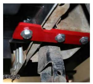
6 Install frame side bumper brackets with the slotted holes facing out and the offset down. Reusing factory bolts, center brackets with slots/holes. The outside width should be roughly 39 3/4".
