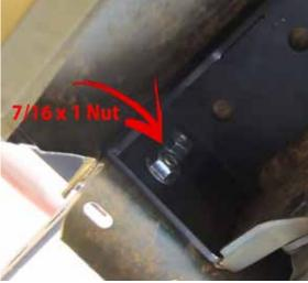
Using a 1/2" drill bit out the two top holes in the spindle reenforcement bracket, see the photo below. You can do this by marking the holes and removing the bracket or by carefully drilling right through bracket.
